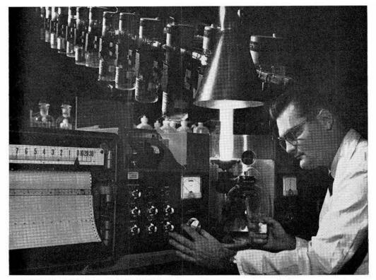
SPECTROPHOTOMETER ANALYZES SOLUTION to determine amount of aluminum contained in liquid sample. H. C. Feemster (8133) is making the analysis. Spare hollow cathode lamps (top center) give the instrument the capability of analyzing 60 or more elements.
